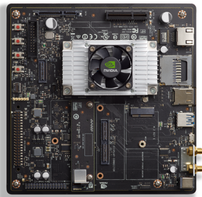
Figure5. NVIDIA Jetson TX2
