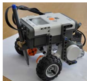
LEGO NXT robot with pen attached to draw Fibonacci spiral
