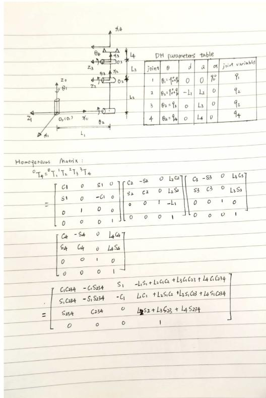
Diagram of a 4-axis robotic arm with DH parameters table and homogeneous transformation matrix derivation.
