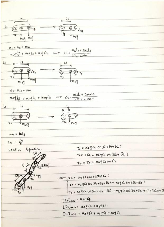
To find capabilities of manipulator with different materials as well as total torque required for motors.
