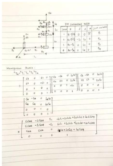
The DH convention was used as shown to find the kinematic solution to this robot. We design a rotation joint in the base, and for the torso of the manipulators we design them as a 3 degree of freedoms planar arms. The DH parameters are as shown above. We multiply each of the
