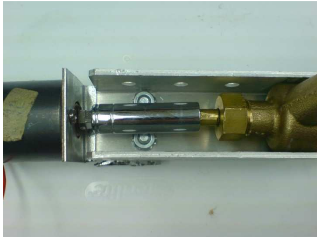
DC Motor-Sprinkler Valve Connection
