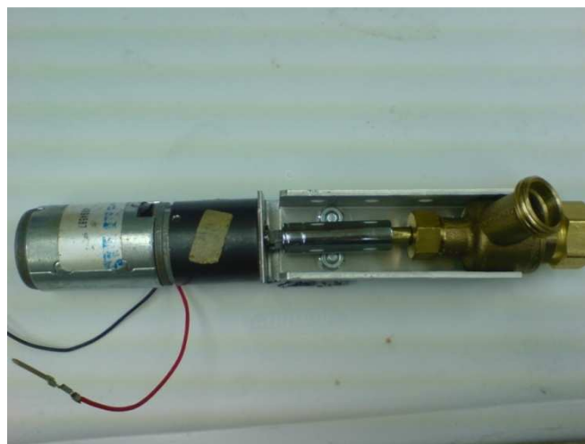
DC Motor-Sprinkler Valve Apparatus
