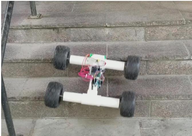
Fig.8 Pet Feeding Robot Stair Case Test
