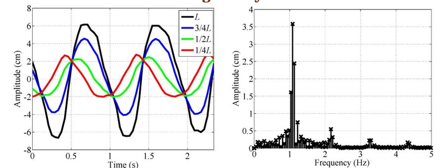
Image analysis was performed using *Xcitet ProAnalyst* to determine the displacement and frequency of oscillation of the realized biomechanical fish tail. Points along the  $1/4$ ,  $1/2$ ,  $3/4$ , and full length of the tail were tracked for a total of 12 periods.
