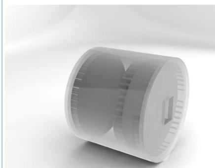
The biomechanical tail is actuated using a water resistant *Hobbico Command CS-80* servomotor. Shown (left) is the computer rendered design of the motor encasement.
