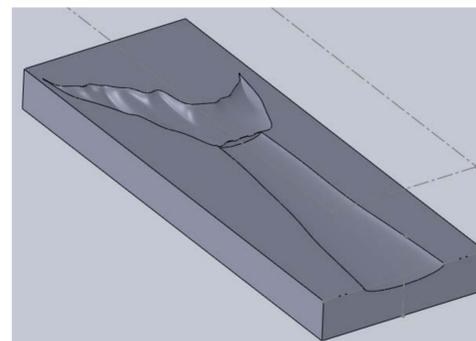
The computer rendered tail section is converted to a computer aided manufacturing (CAM) geometry, shown (right). A slender stainless steel beam is inserted into the mold for structural support.
