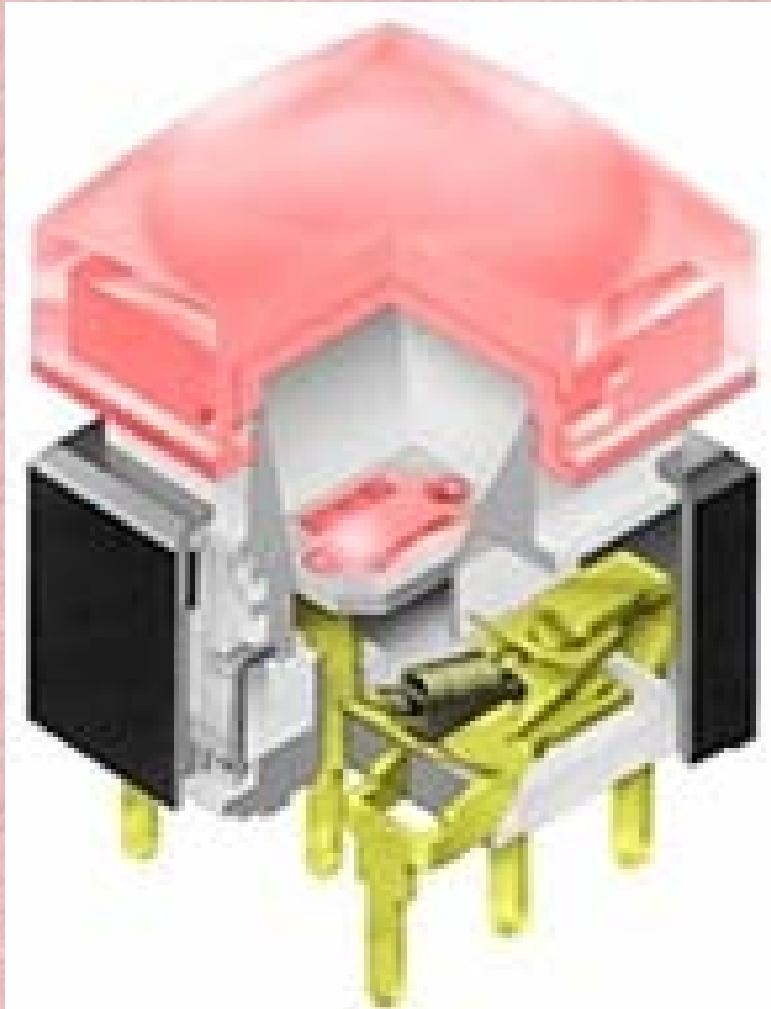
A push button is a device that connects wires to complete a circuit thus allowing current to flow
