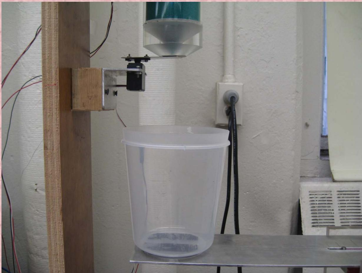
A servomotor is an electrical motor that produces rotation of less than a full turn
