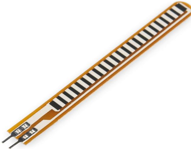
Inside the flex sensor there are carbon resistive elements within a thin flexible substrate. When the substrate is bent, the sensor outputs a resistance relative to the bend radius. The nominal resistance value of the flex sensor when it is straight is  $15\text{K}\Omega$  to  $22\text{K}\Omega$  when it is bent to  $90^\circ$  angle.
