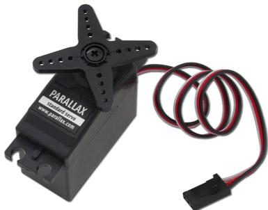
There are two kinds of servo motors, e.g. continuous servo and standard servo. Standard servo has only angular motion of 180°. Continuous servos, as the name suggests, can provide a continuous rotary motion. That is why continuous servos are used to impart motion to our Boe-Bot(wheelchair). The speed of the servo motor is controlled by a method called Pulse Width Modulation.
