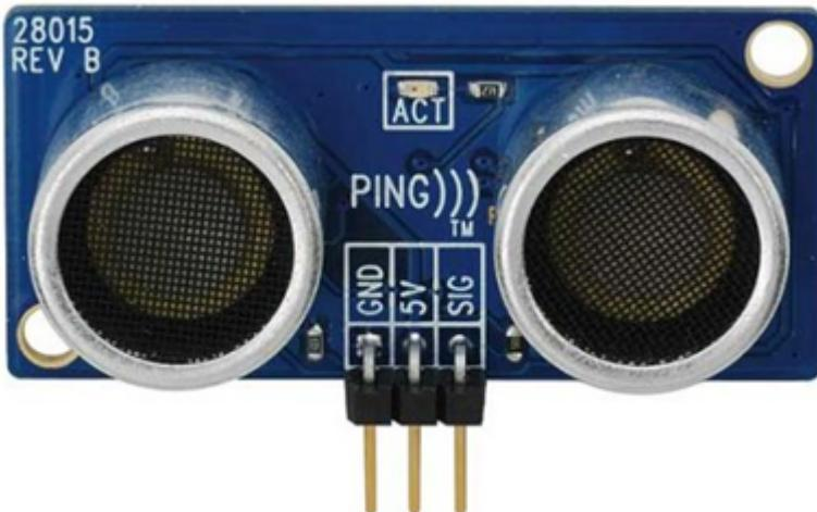
The ping sensor provided by parallax is used as a front obstacle detector
