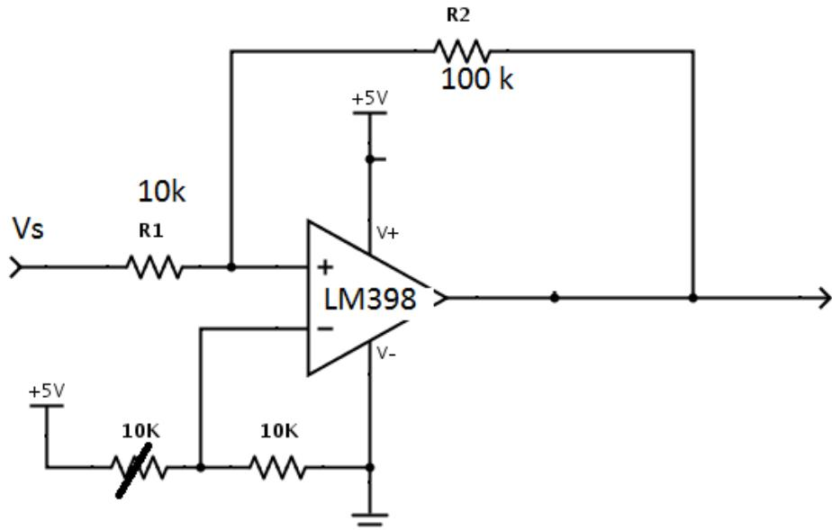
The OpAmp compares the IR analog voltage to the pot voltage to check if cliff is present
