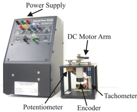
Figure 2: DC motor test-bed
