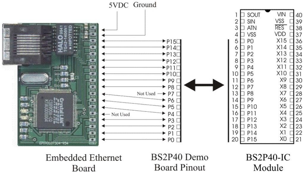
Figure 4: Pin connections between the EEB to BS2P40
