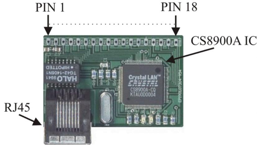
Figure 3: The embedded ethernet board
