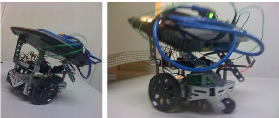
A web-enabled robot prototype, based on the Parallax Boe-Bot robotics kit, with a mounted wireless router and Parallax Internet Net burner Kit (PINK).
