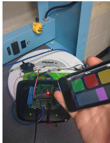
The iRobot with a Linksys wireless router and MAKE controller mounted on it for OSC capability over a Wi-Fi network.
