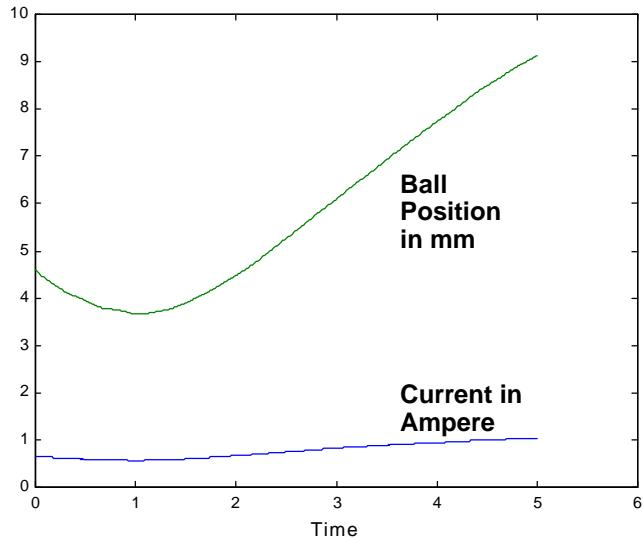
and the current when the ball is tracking a slow sine wave.
