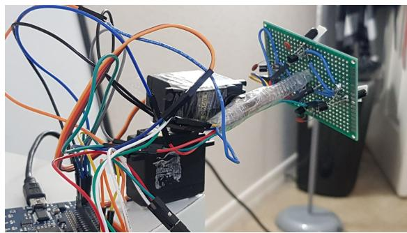
To it PCB board with sensors is soldered to it. The sensors are oriented in such a way that there are three in each axis.
