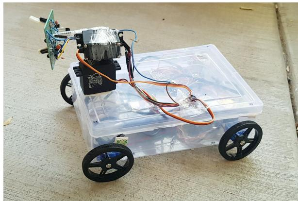
A PCB board with a battery, arduino nano, buzzer soldered to it along with the Raspberry Pi with all the required connections is placed inside the box. The whole setup is powered by a power bank which is also placed inside the box.
