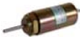
**Pull Solenoid.** This is an electromagnet device consisting of a coil of wire called a solenoid and an iron plunger inserted partially inside the solenoid. When current flows through the solenoid, it produces a magnetic field just as a bar magnet. This magnetic field pulls then plunger. The strength of the solenoid's magnetic field is dependent upon the amount of current flowing through it.
