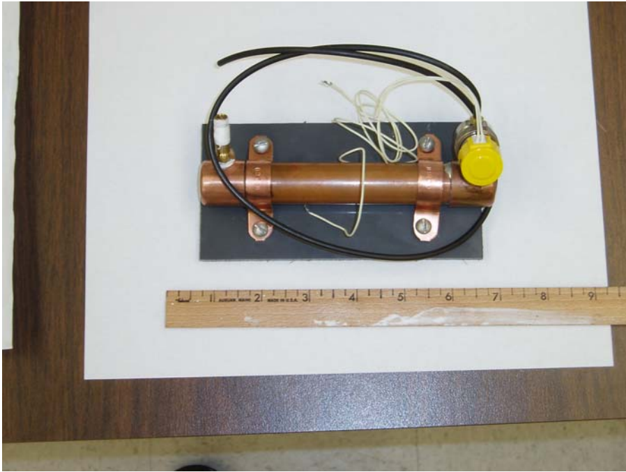
Compressed Air Tank
