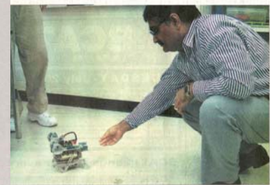
Prof. Vikram Kapila of Polytechnic University demonstrates this robot with military sensors in its "ears," amplified by paper cups.
