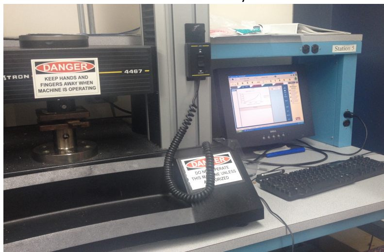
Figure: Quasi-static compressive testing
