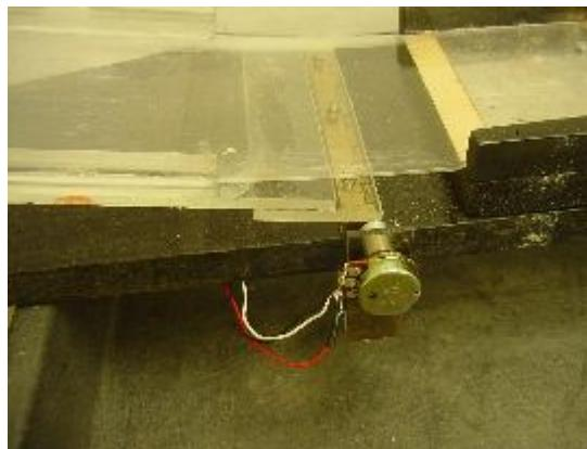
After the user inputs an angle, the Basic Stamp compares the input angle to the actual angle of the platform. The dc motor begins to raise the platform.
