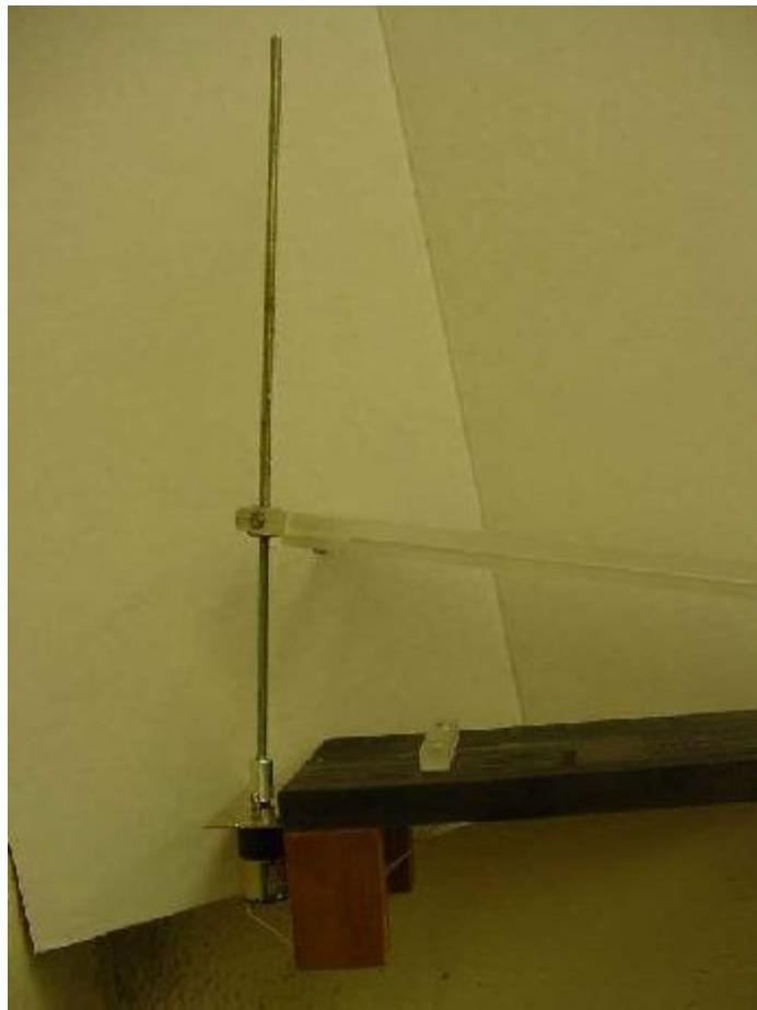
As the cart comes down it interrupts two photogates which consists of an Infrared Emitter Diode and a Phototransistor. The the cart travels along the track and interrupts the photogates, sending a signal to the Basic Stamp
