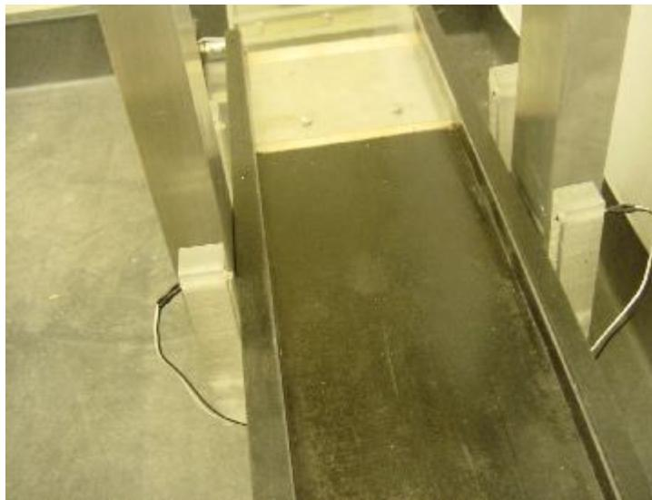
After it passes the photogates the velocity of the cart is measured. A delay time is calculated. At the proper time the push solenoid activates and launches the ping pong ball off the launch platform.
