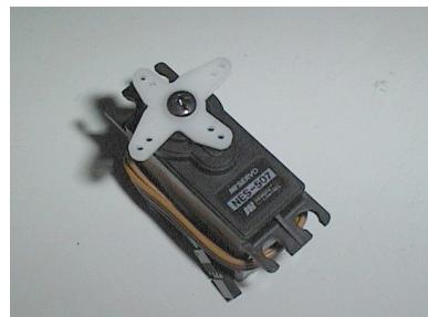
**12 volts DC motor with reduction gearing** – Provides the work to raise or lower the incline. The motor is geared down to increase torque and decrease angular velocity
