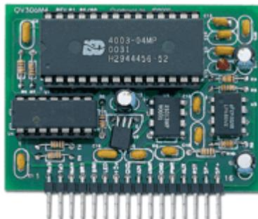
**1 ADC Converter** The Analog to Digital Converter converts an analog potential to a digital signal which can be interpreted by the Basic Stamp
