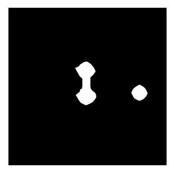
The software filters brought down the minimum Euclidian distance between two robots to be 15 cm. Another layer of hardware polarized filter was aded to the camera lens as an experiment to improve performance.
