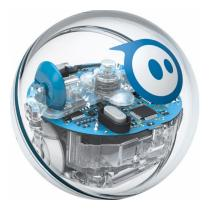
Spheros is by configuration a differential drive robot placed inside a sphere. The company provides ros packages and general api's that allow developers to connect with a sphero. The Sphere has 2 bright multicolored LED's, used Bluetooth as mode of communication and has a built in IMU based stabilizer.
