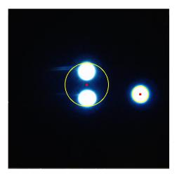
As the distance between two robots is less than 15cm, two individual blobs fuse to look like one huge blob. This limits the number of robots on the arena and the range of motions possible.
