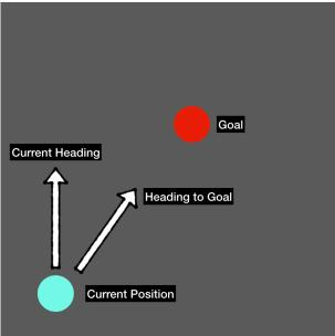
The velocity 'V' of the robot is chosen proportional to the distance error and the angle error is used to calculate the angle steps  $\Delta$ Theta.
