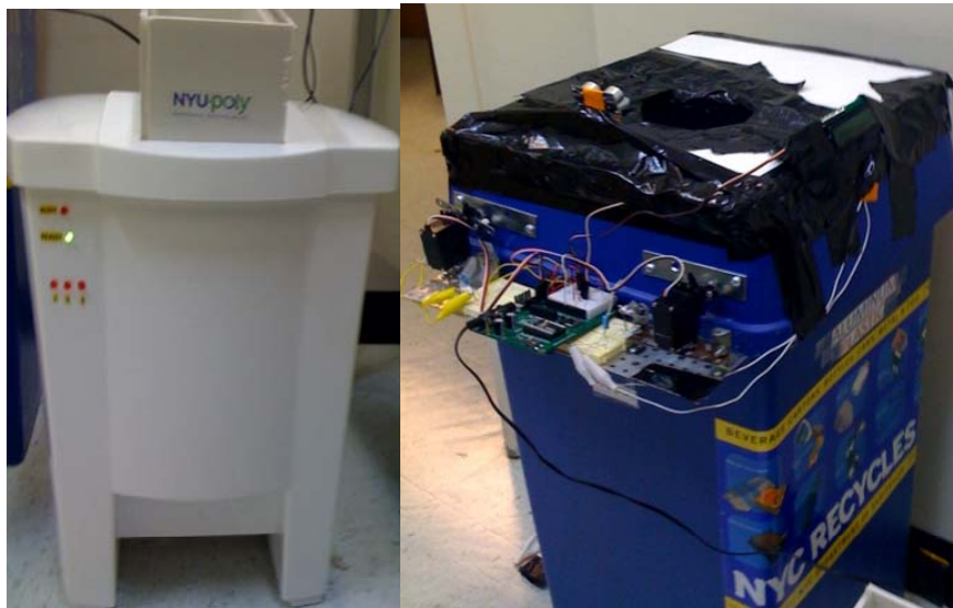
Figure 1: a) Trash can which sorts trash based on their dielectric constant with capacitance sensors, b) Trash can which sorts trash based on light interaction.
