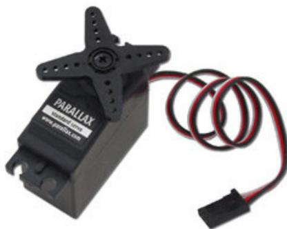
The vertical servo will range an angle of approximately  $157.5^\circ$  and will move left to right from the position 1000 to 250 and the other way round right to left from 250 to 1000. The horizontal servo will move up and down from the position 1000 to 550 and backwards.
