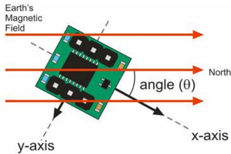
Of course if the  $x$  component is maximum and the  $y$  component is null, the compass is facing the magnetic north otherwise the angle  $\theta$  is given from the relation
