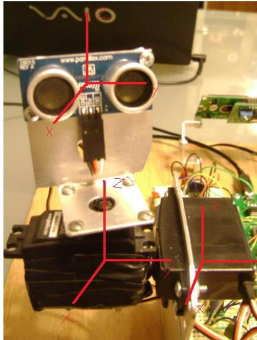
The frame attached on the Ping will be named  $x'y'z'$ , the one attached to vertical servo  $x''y''z''$ , while the one that is fix and attached to the base will be  $xyz$ .
