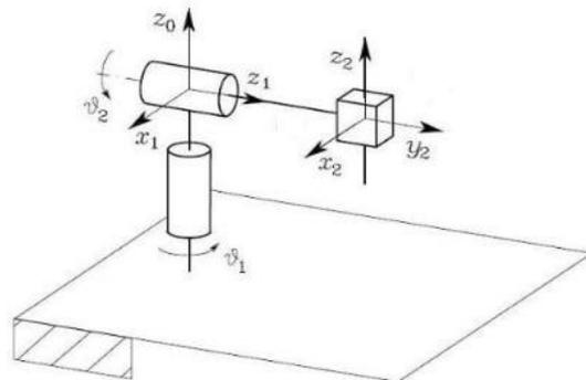
So, the two angle  $\vartheta_1$  and  $\vartheta_2$  are the one swept by the servos, while we can see the little cube as the Ping sensor mount on the second servo. Our target will be moving on the frame of reference attached to the Ping sensor while the position outputted by the algorithm has to be the one relative to the frame of reference attached to the solid base.
