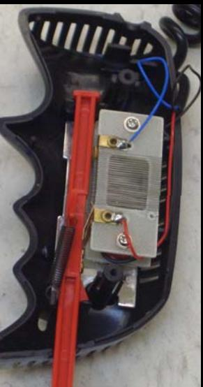
This is the controller that came with the car set. It is essentially a "push-button" mechanism that slides along a path of different resistances which control the car speed.
