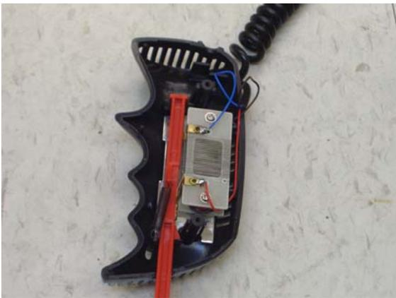
discovered that the inside consisted of two approximately two inch long resistors. The resistor on the left was connected to the live wires. The resistor on the right was connected to ground. The push-button has a shaft with a small metal piece attached. As the push button is held down, the metal piece slides down the resistors, making a connection between the two
