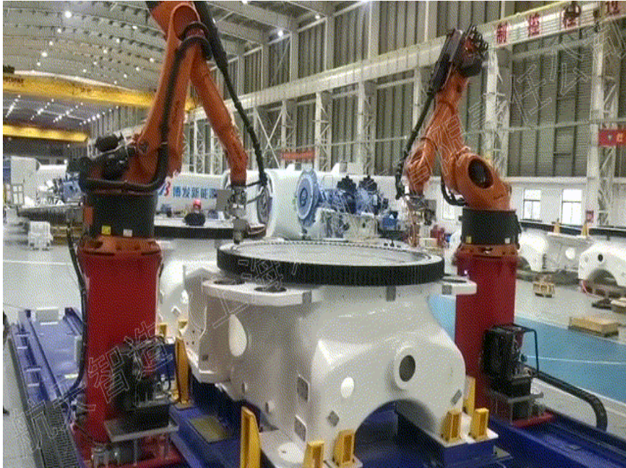
Yunda wind power production site: The hub bolt fastening robot system
