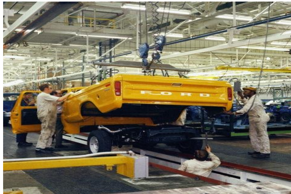
1973: Placing an F-Series bed onto the frame
