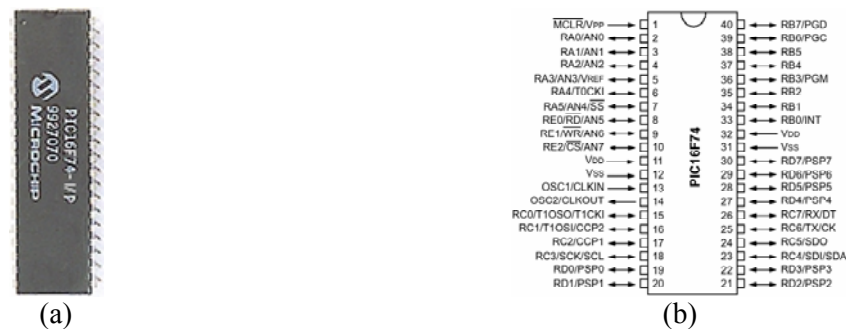
Figure 1: (a) PIC16F74 (b) Pin diagram of PIC16F74
